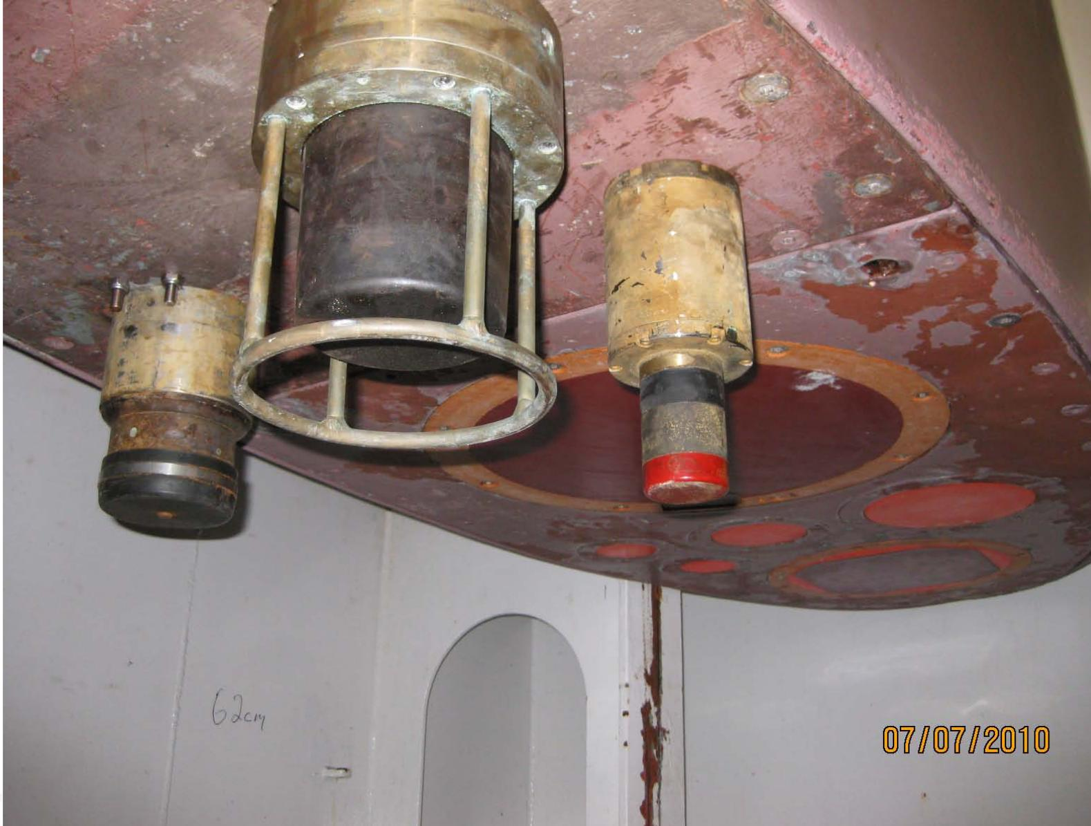
Hydrophones for commands and data communication installed in drop keel.
